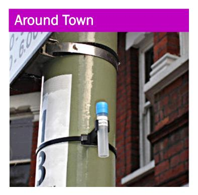
You may see some odd bits of equipment attached to lampposts and street signs. These are passive monitoring devices for nitrogen dioxide gas. These are exposed for approximately one month and swapped on a given date for another, year round. The tubes are sent to a laboratory which determines the nitrogen dioxide concentration at the tube's location for the period it is exposed. They are installed by NCC as part of our their requirements to monitor and report on air quality within Northumberland.
